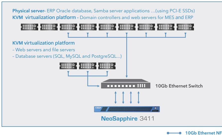
Figure 1 : Architecture diagram of Topkey adopting NeoSapphire 3411 to their virtualization platform
